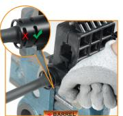
Place the Barrel Nut Wrench in the second slot on the Barrel Nut (closer to the receiver). NEVER USE THE FIRST SLOT TO TIGHTEN. Warning: Max. torque value for installing barrel nut should not exceed 60 ft-lb.
