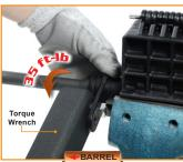
Use the Barrel Nut Wrench to securely tighten the Barrel Nut with enough tension (35 ft-lb.). (We recommend using a torque wrench to achieve proper tension).
