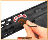
Once you achieve the proper alignment of the threaded holes on the Locking Ring to those on the handguard rail, use the T20 Torx Wrench and 6 of the Locking Torx Screws to securely lock the handguard to the Barrel Nut/ Locking Ring assembly.
