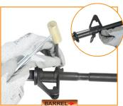
Securely place the barrel on a well padded flat surface. Using a hammer and punch, tap out the two pins at the bottom of the front sight/ gas block. Remove the front sight/gas block, the gas tube, and front handguard cap.
