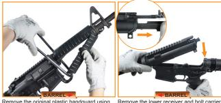
Remove the original plastic handguard using the handguard removal tool.
