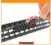
Once the Rail Section is seated properly, use the included 3/32" Hex Wrench to hand-tighten the screws on top of the Picatinny Rail Section to lock it securely to the Keymod Compatible Handguard. Do not over-torque.
