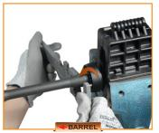
Clamp the upper receiver on a vise with an AR15 upper receiver vise block. Loosen the barrel nut by turning it counterclockwise with an AR15 barrel nut wrench. Remove the original barrel nut and delta ring assembly.
