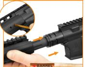
Carefully slide the handguard over the Barrel Nut/Locking Ring assembly. Make sure there is a positive connection between the top rail of the handguard and the top rail of the receiver (there should be NO gap here). If you lose the alignment of the Locking Ring, use your Hex Wrench to realign the threaded holes.
