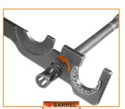
Remove the flash hider by turning it counterclockwise with an AR15 combo wrench.
