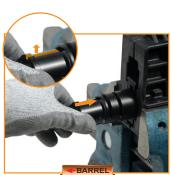
Slide the Locking Ring into the Barrel Nut, making sure the alignment slot on the Locking Ring is vertical and facing upward.
