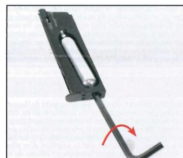
Tighten the screw located on the magazine. When pressure starts increasing in the magazine (expansion of the CO2 in the magazine can be heard), finishing screwing rapidly. Very important: do not tighten excessively, it could permanently damage the O'rings.
