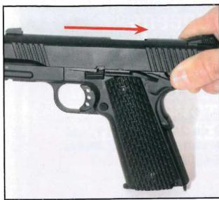
• In order to fire, you have to cock the gun : pull the slide backward as shown and release.
